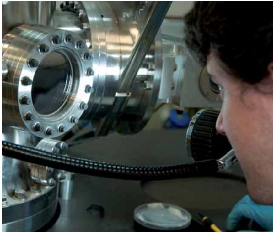
INSTALLED IN THE LABORATORY FOR SURFACE ENGINEERING, THE PHOTOELECTRON SPECTROSCOPY EQUIPMENT PERFORMS THE CHEMICAL ANALYSIS OF MATERIALS WITH HIGH PRECISION
