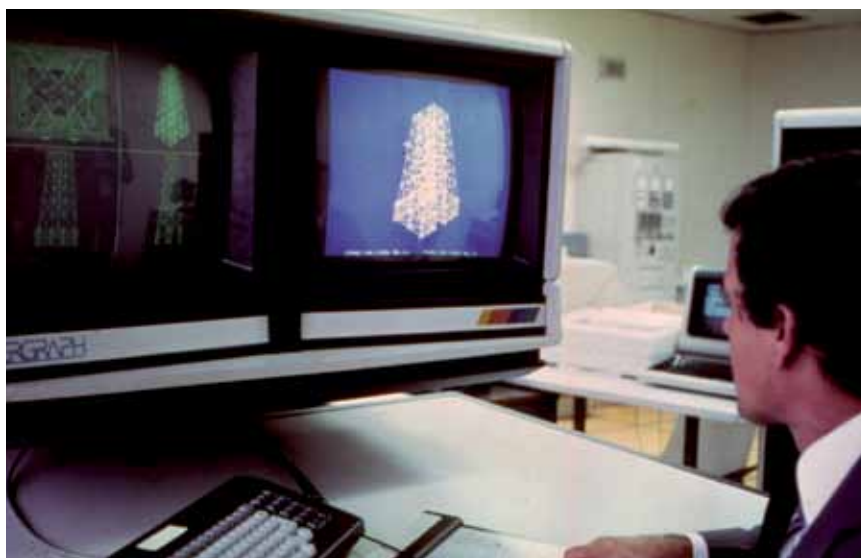
A RESEARCHER OF CENPES USES A SISPLLOT VISUALIZATION MODULE OF THE ADEP (ANALYSIS AND MEASUREMENT OF STRUCTURES AND PLATFORMS) AND INPLA (PLATFORM INSTALLATION) SYSTEMS DEVELOPED AT COPPE IN 1977, FOR OFFSHORE PLATFORM PROJECTS AND INSTALLATIONS
